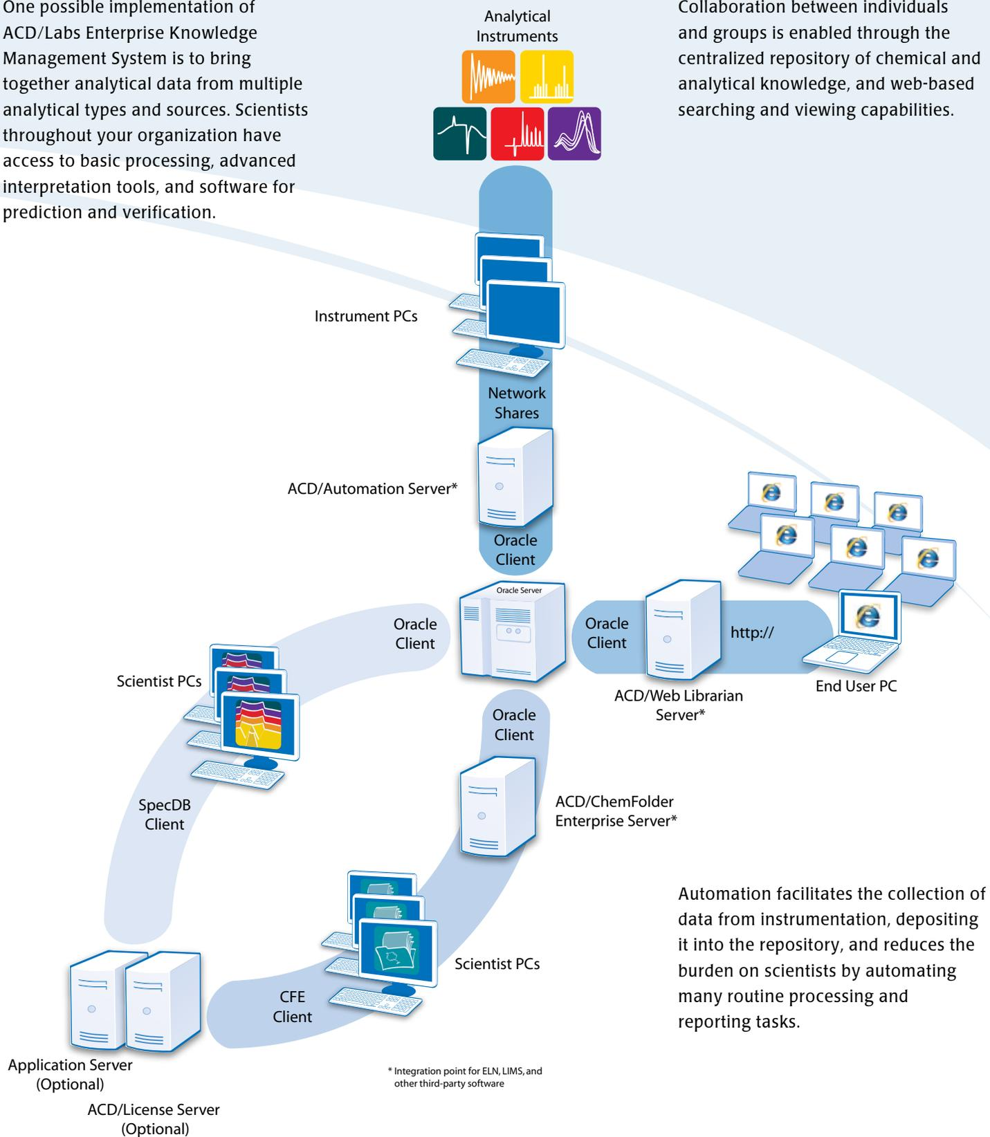
Automation facilitates the collection of data from instrumentation, depositing it into the repository, and reduces the burden on scientists by automating many routine processing and reporting tasks.
