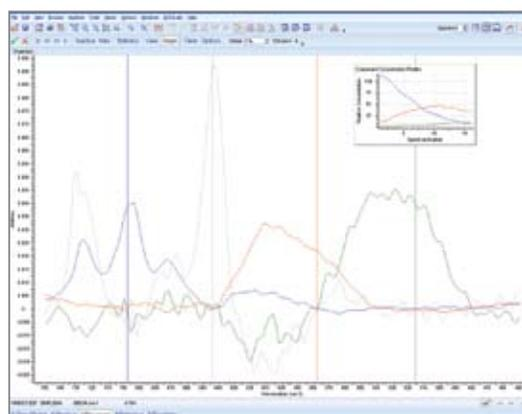
Resolve pure components from a series of spectral mixtures and obtain corresponding concentration profiles with SIMPLISMA (SIMPLE-to-use Interactive Self-Modeling Mixture Analysis). This highly interactive curve-resolving algorithm extracts individual components without requiring *a priori* knowledge of the mixture composition.
