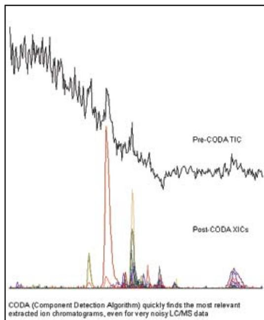
CODA (Component Detection Algorithm) quickly finds the most relevant extracted ion chromatograms, even for very noisy LC/MS data
